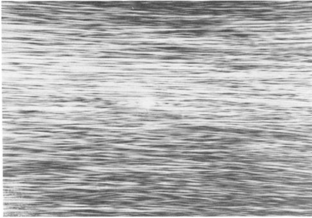
FIG. 9—The H_v pattern of wool fiber suspended in air (fiber axis vertical).
